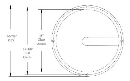
\* Stainless Steel Hardware & Gasket Tape For Gas Tight Seal Provided
