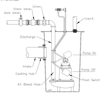
Pump can be installed with ABS, PVC, polyethylene or galvanized steel pipe. Proper adapters are required to connect plastic pipe to pump.
