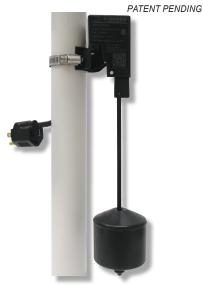
The VertiMAC™ is a float operated pump switch, typically used in sump pump applications or situations where a regular pump switch cannot operate due to limited space. Available in 120VAC or 240VAC, bare lead (no plug) or piggyback plug, 13 Amp models.
